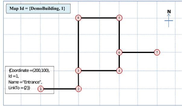
Fig. 2: A graph representing a level of a building
