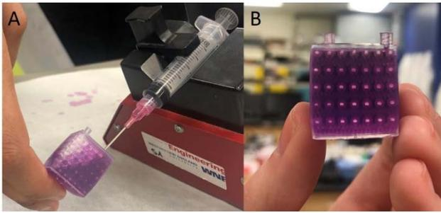
Fig. 2: (A) Device testing in the class using a syringe pump and food color. A mathematical formula was used to assess the success of the design. (B) Student holding their 3D printed scaffold after completion of the test.
