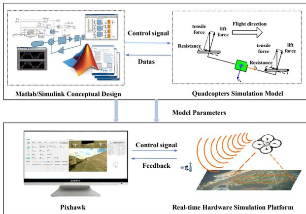
Fig.4. Conceptual Design and Simulation
