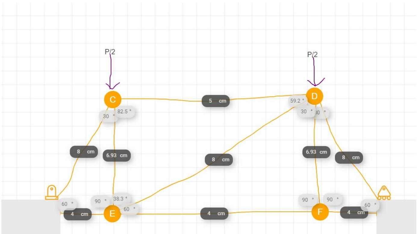
Figure 2: Example of Mechanics User Interface, with a drawn Truss system. This example comes directly from the Truss Design Mode, in which students are given freedom to develop their own solution to an open-ended question, in which they have to meet certain specifications set by the instructor while attempting to maximize the load that the truss can take.
