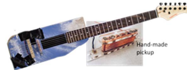
Fig. 1. An electric guitar resulting from a designette in an advanced physics course. The designette of 1D Big-D requires students to use Faraday’s Law and the wave concept in physics to make a simple electrical guitar.
