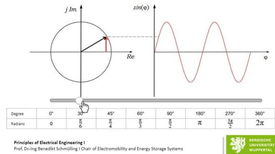
Fig. 3. Complex numbers and unit circle in context of alternating voltage
