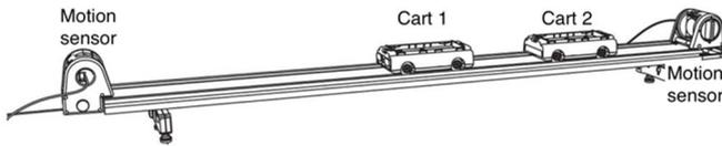
Fig. 5. Experimental setup for the impulse and collision lab
