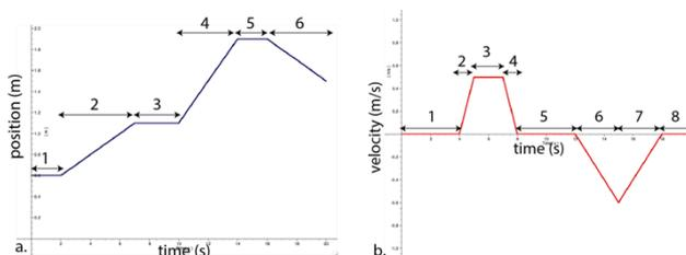
Fig. 3. Illustration of a *position-time* (a) and *velocity-time*-graph (b), that students are requested to match by their own movements in front of a motion sensor (Fig. 2). To facilitate analysis the different sections of the graphs are numbered. However, they are not numbered in the task students' participate in.
