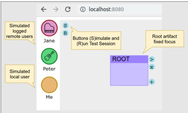
Fig. 6. Prototyped workspace and testing resources.
