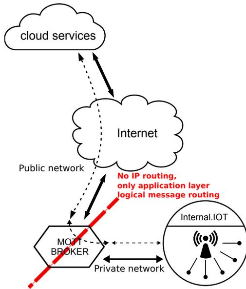
Fig. 7. VREL Security: MQTT routing model
