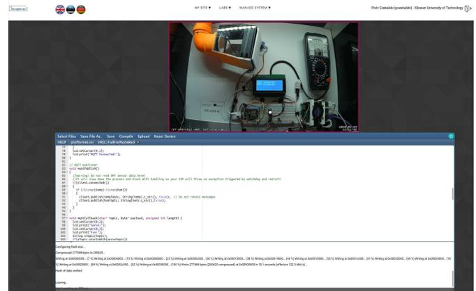
Fig. 2. User interface for the end node programming in C++
