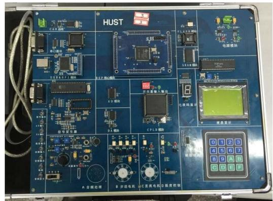
Fig. 6. University self-developed DSP platform.
