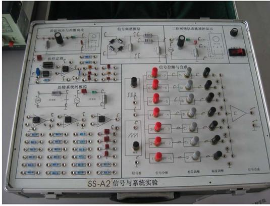
Fig. 5. A lab box of signal processing hardware circuit.
